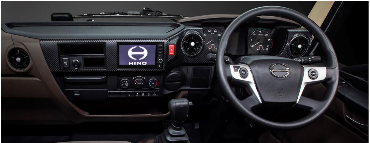
Example of Directed Technologies OE Australian designed in-vehicle 'factory' navigation driver alert system which is designed for the vehicle with appropriate GUI / HMI including steering wheel control integration, voice distraction free alerts, speed relevant HMI control etc. The system has tyre pressure monitoring and alert, seatbelt and park brake alarm, reversing and lane change cameras and a wireless phone charge pocket to encourage phones to be paced out of reach and out of view. Phone calls are able to be managed by the driver via the steering wheel controls and voice recognition. Copyright Directed Electronics and HINO Australia.
