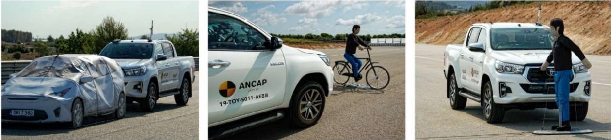
Figure 2 - AEB Scenarios: Car to car rear, Car to adult cyclist and Car to pedestrian
