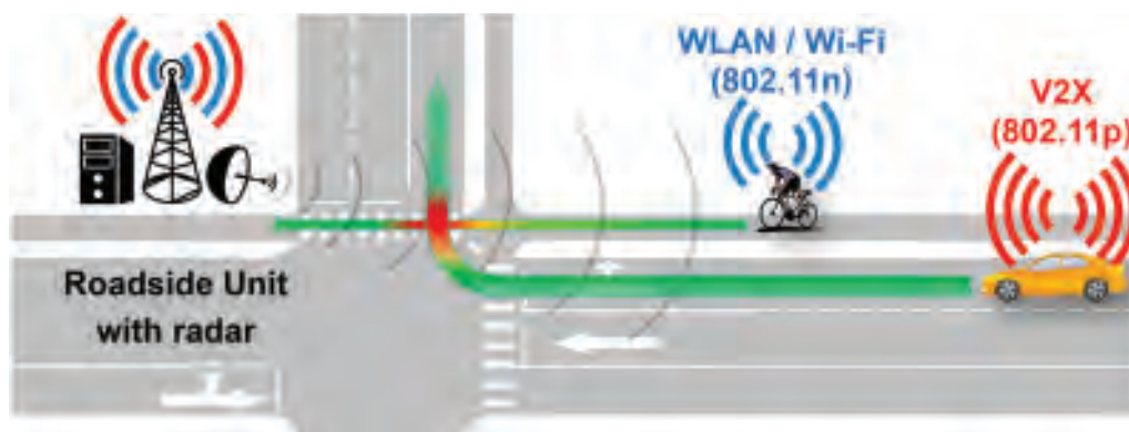
Figure 9. Conceptual collision prevention for connected vehicle and cycle with roadside radar interaction, Tim Russ, ifak (23rd World Congress, Technical Session 23)
