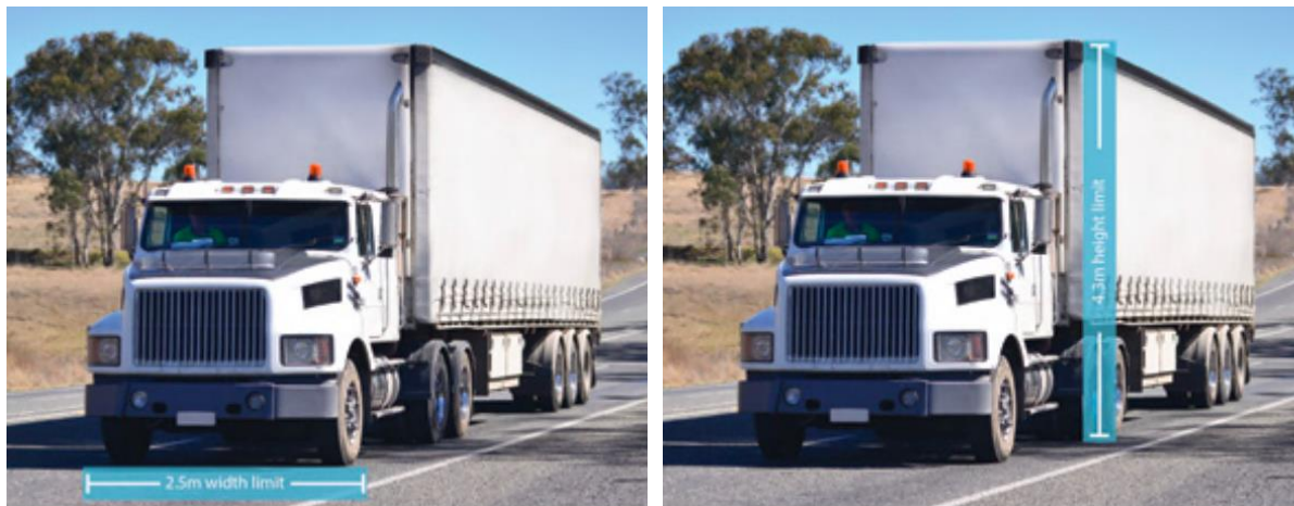
Heavy vehicle 2.5 metre width limit
