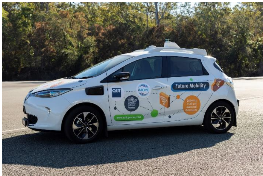
Figure 2: ZOE2, a research prototype connected and automated vehicle (CAV) developed by Queensland's department of Transport and Main Roads in partnership with Queensland University of Technology and VEDECOM research institute, France.
