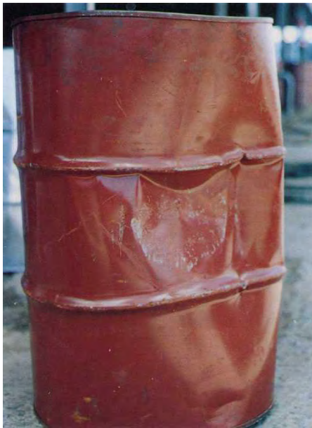
Figure D1: Reprocessing steel drums – dents
