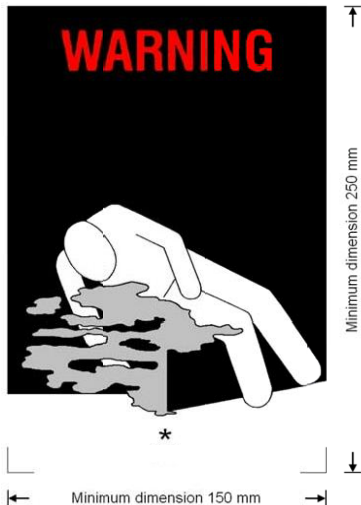
Figure 5.5.2: Asphyxiation warning mark for cargo transport units
