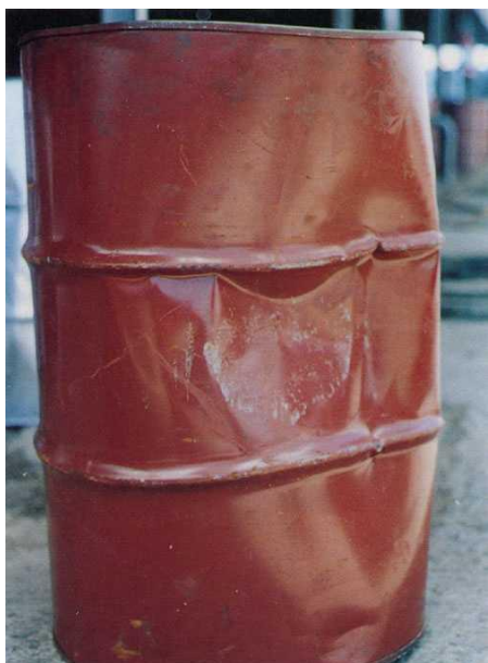
Figure D1: Reprocessing steel drums – dents
