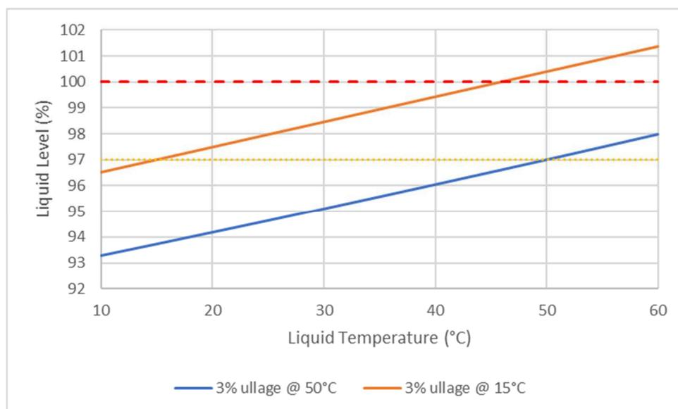
Note: this figure uses a thermal expansion coefficient of 0.001 K<sup>-1</sup>.
