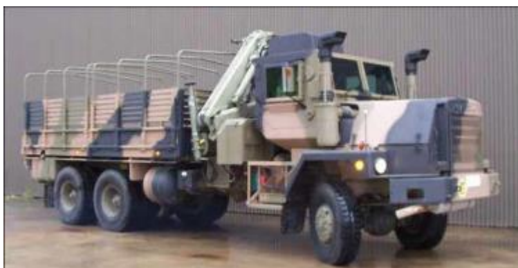
Figure 5-19 – Mack Up-armoured variants (armour protected cabin)
