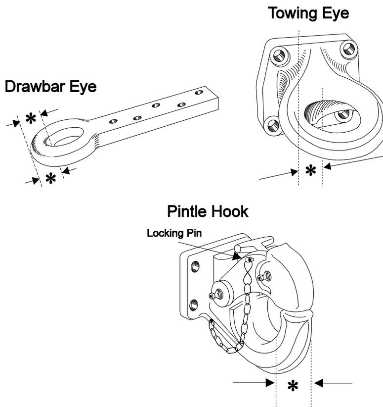
*Note: If a section reduction is visible when the eye and coupling are connected, this wear condition is likely to exist.*
