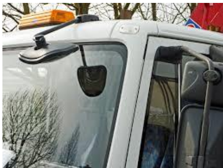
Example of a class VI mirror fitted to a heavy vehicle (note – left hand drive)
