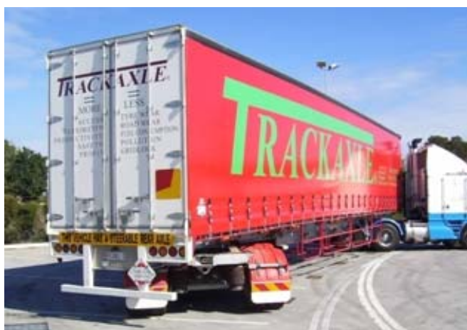
Figure 3. Example of a SMART vehicle, with steerable rear axle, that may operate under the PBS scheme.
