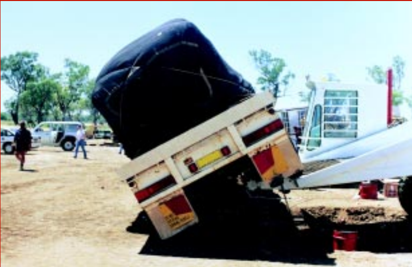
Cotton module tilt test in side direction.
