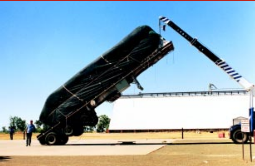
Cotton module tilt test for rearward and forward direction.
