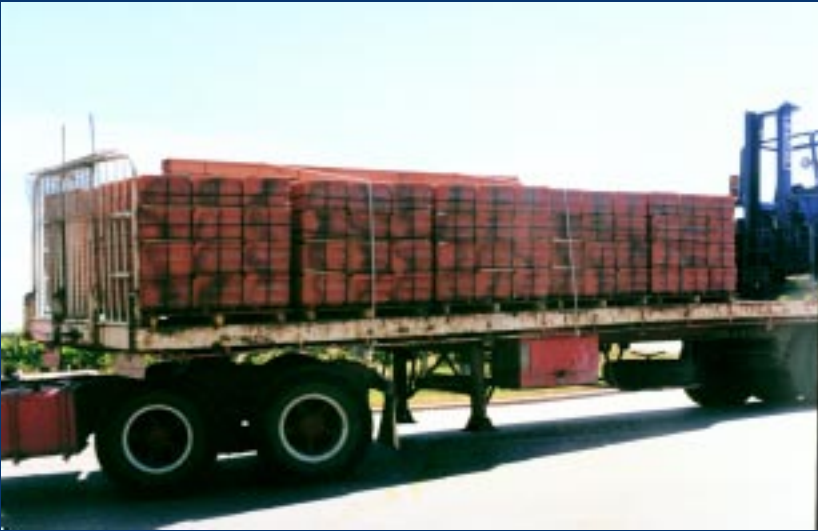
Two ropes and the pipe loading rack in front won't restrain this load of tiles and batters.
