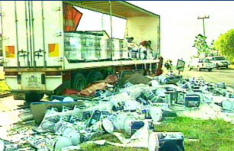
The side curtain could not restrain these pallets of cooking oil.
