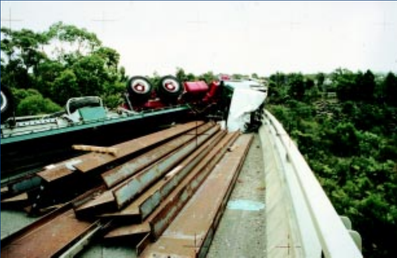
Poor load restraint caused the heavy steel sections to move and cause the rollover.
