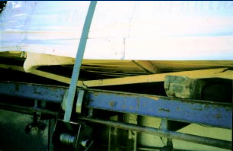
The base of the load broke from the strapping tie-down force. The strap should have been positioned above the dunnage supporting the load. (Photo courtesy Queensland Transport).
