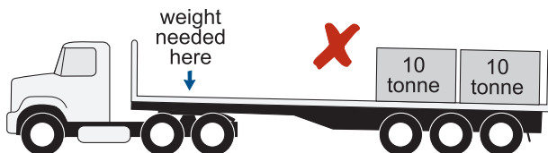
Fig. B.10 INSUFFICIENT WEIGHT ON DRIVE AXLES
