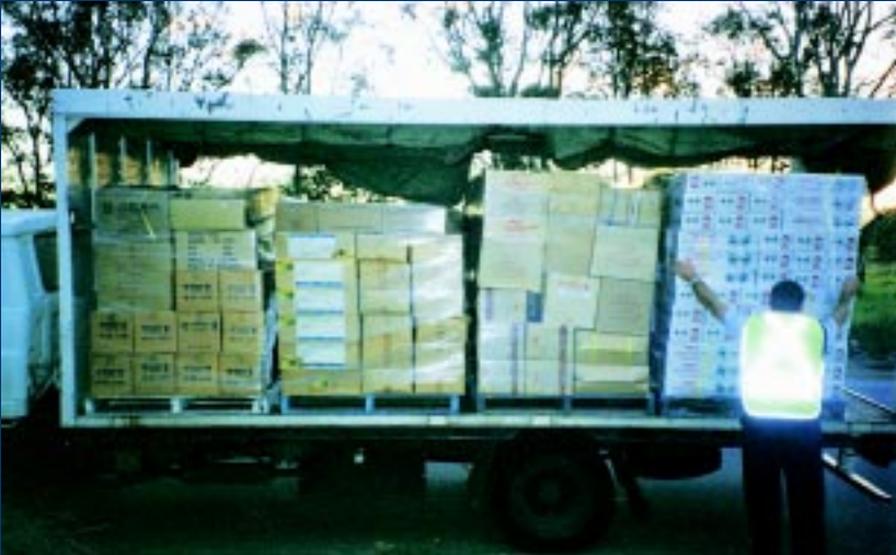
There were no lashings on this load and the plastic wrapping did not adequately hold the load together. (The enforcement officer is holding a leaning pallet of boxes on the truck while the driver is getting some restraint equipment from the toolbox).
