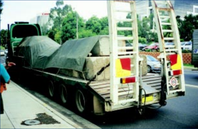
A tarpaulin alone cannot restrain this load of concrete blocks.
