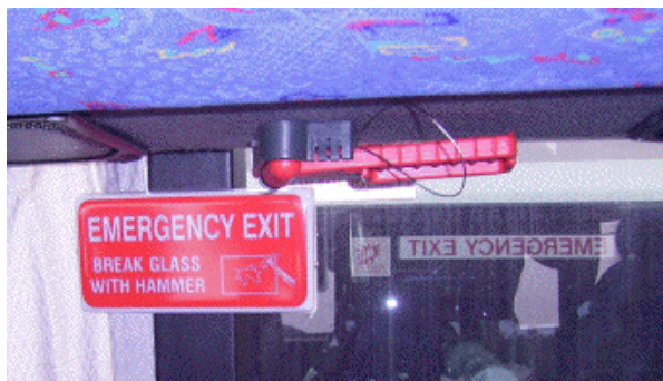
Figure 5. Example of 'break glass' installation
