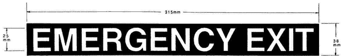
Primary "Emergency Exit" sign
