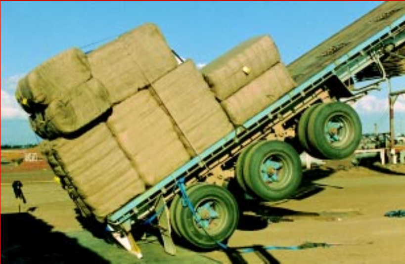
Tilt testing a cotton bale packing arrangement.
