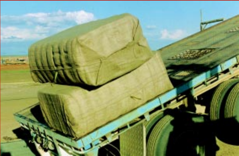
Testing the friction by tilting the load and measuring the angle at the point it just slides. The test is for both the friction between the bales and the bales and the deck.
